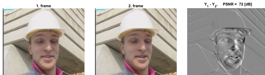
Figure 4.2: Adjacent image in video stream (a-b) and the difference of the luma matrices (c).
