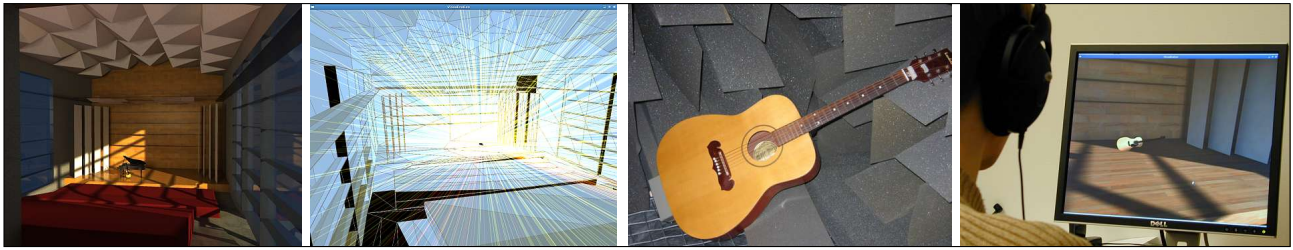
Figure 1. The acoustics of a concert hall model is simulated with the acoustic radiance transfer method. The results from all the surface patches are convolved in realtime with an anechoic stimulus to create a binaural interactive auralization.
