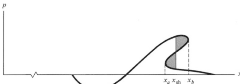
Fig. 11.5 The equal-area rule for determination of the location of a shock; the two equal shaded areas are replaced by a discontinuity in the waveform
