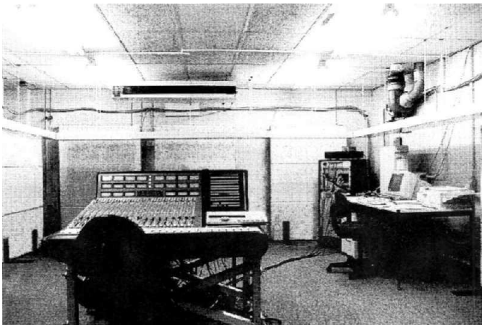
Figure 4.12 The laboratory reproduction room with the mixing console (left), the arrays (nos. 3 to 6), and the DSP-system (in the corner of the room).
