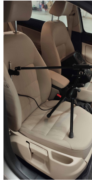
Figure 2: Measurement of surface impedance with a Microflown PU-probe
