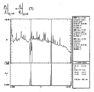
Figure 1: in-flight noise spectrum and right-engine coherence
