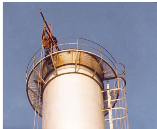
Photo 2. Mounting of the microphone for near-field measurement at the stack opening
