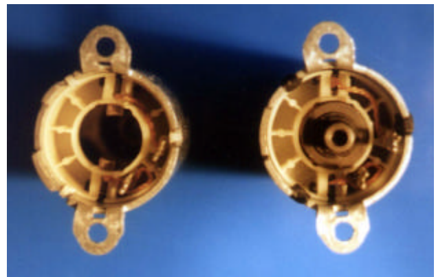
Figure 7. Front view of the motor (plastic bearing holder removed). Left: positioning studs weakened but still naked, right: studs isolated + rotor inserted.
