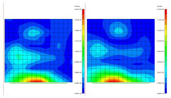
Fig. 2. Comparison of sound pressure fields of the tire at 722 Hz: direct measurement (left) and I-BEM calculation (right)
