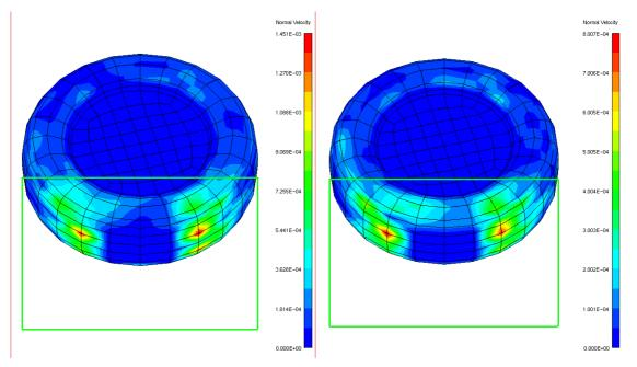
Fig. 1. Calculated velocity distribution along a tire at 722 Hz with TSVD (left) versus Tikhonov (right) regularisation
