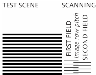
Figure 6.6 Twitter would result if this scene were scanned at the indicated line pitch by a camera without vertical filtering, then displayed using interlace.
