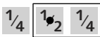
Figure 10.5 Cosited chroma filter for Rec. 601, 4:2:2 causes each filtered chroma sample to be positioned coincident – cosited – with an even-numbered luma sample.
