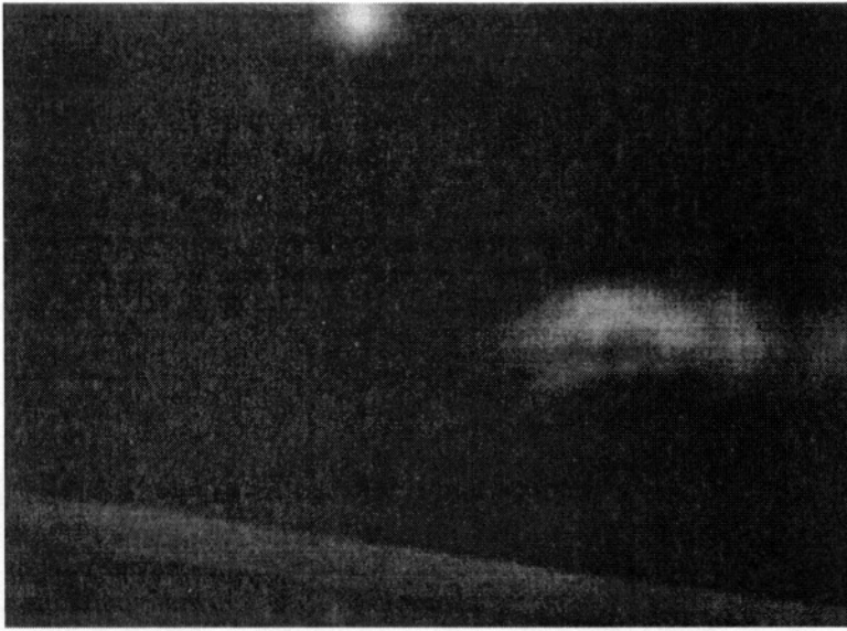
Figure 13.5: Mean average distortion over a 256x193 pel search range for a macroblock from a picture in the table tennis sequence. The example was generated for macroblock (10,10) in picture 6, with prediction from picture 2. A blurred hand holding a paddle is clearly distinguishable. Darker areas have lower MAD.
