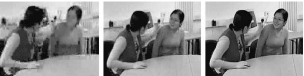
Figure 4.23 A video frame compressed at the same bitrate using MPEG-2 (left), MPEG-4 Visual (centre) and H.264 compression (right)
