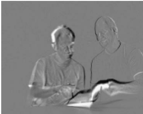
Figure 3.12 Residual : no motion compensation
