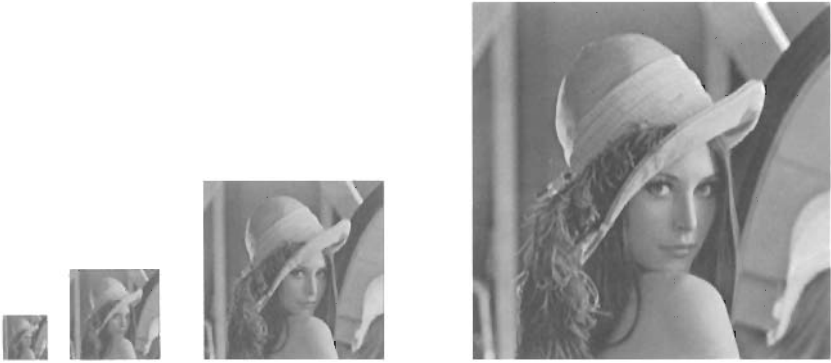
FIGURE 7.23 Multiresolution approximations a_j[n_1, n_2] of an image at scales 2^j , for -5 \geq j \geq -8 .
