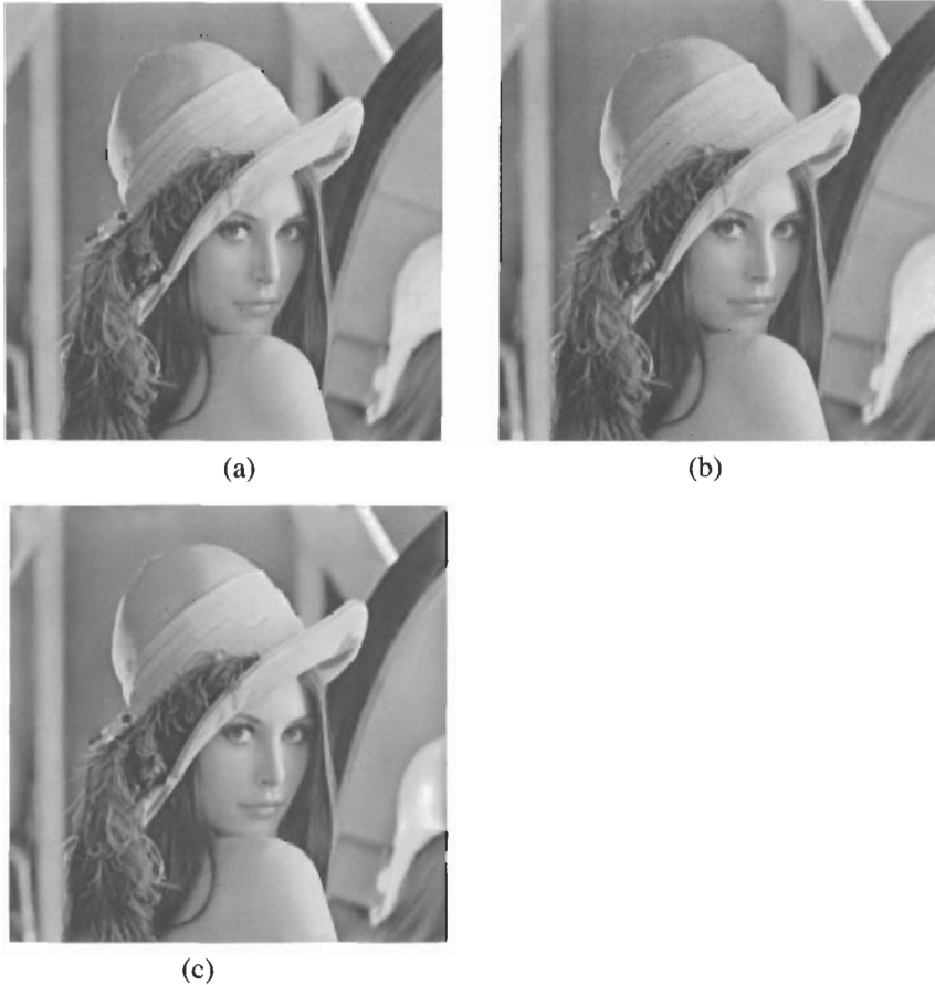
FIGURE 6.11 (a): Original Lena. (b): Reconstructed from the wavelet maxima displayed in Figure 6.10(e) and larger scale maxima. (c): Reconstructed from the thresholded wavelet maxima displayed in Figure 6.10(f) and larger scale maxima.
