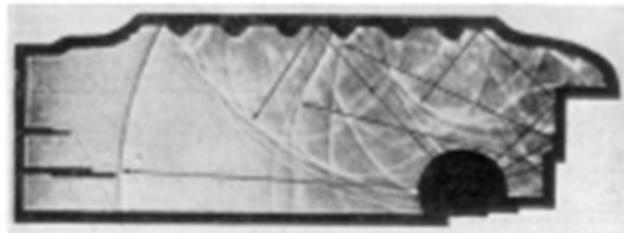
Fig. 1. Schlieren photograph showing reflections of ultrasound wave fronts in a sectional model of the Gewandhausaal in Leipzig. (Teddington – from Engl, [2]).
