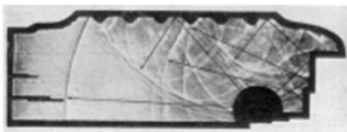
Fig. 1. Schlieren photograph showing reflections of ultrasound wave fronts in a sectional model of the Gewandhausaal in Leipzig. (Teddington – from Engl. [2]).
