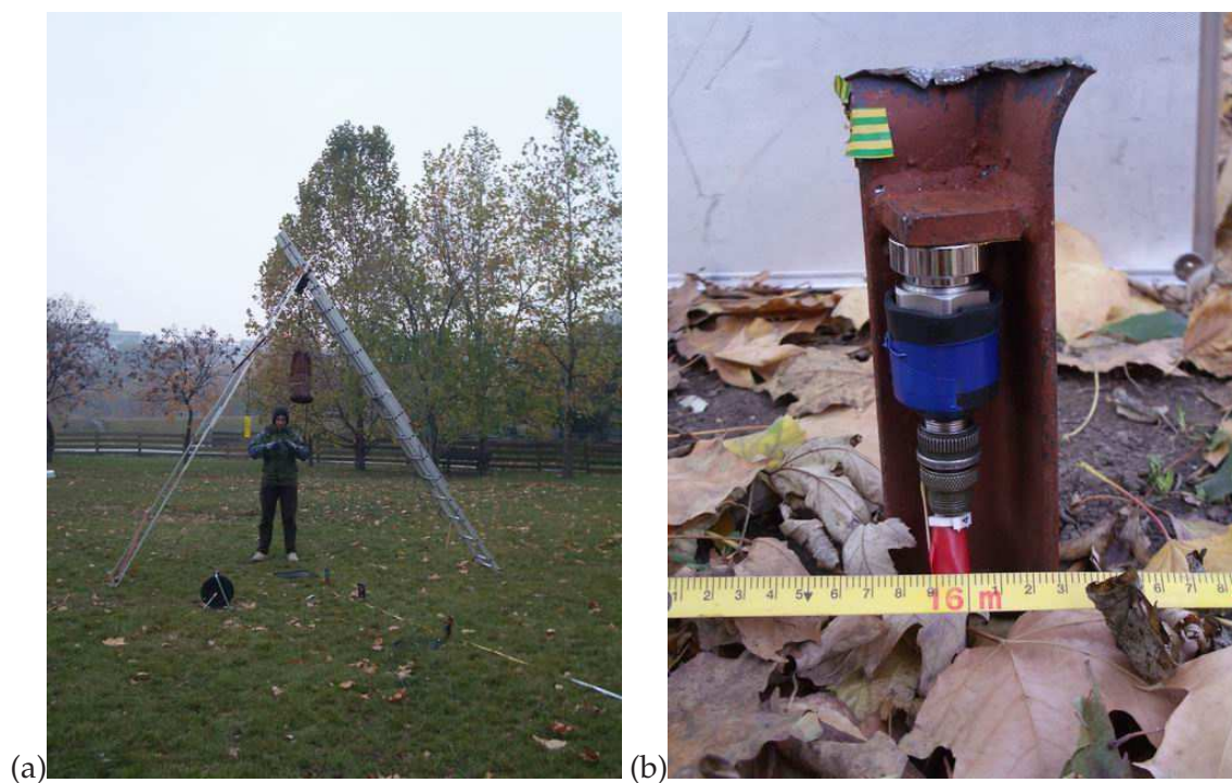
Figure C.2: The measurement setup: (a) 80 kg heavy bang filled with lead shot, (b) PCB 393A03 acceleration sensor mounted on a steel pike.
